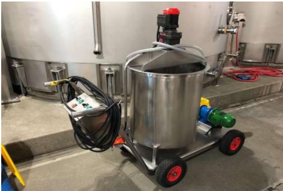
Figure 7. Mobile tank and mixer for making up additives in winery, complete with transfer pump.
