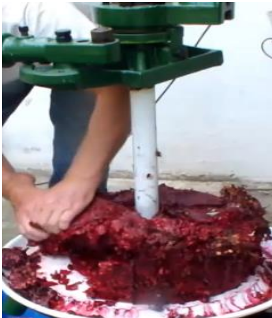
Figure 23. Remove break down press cake and collect in to container
